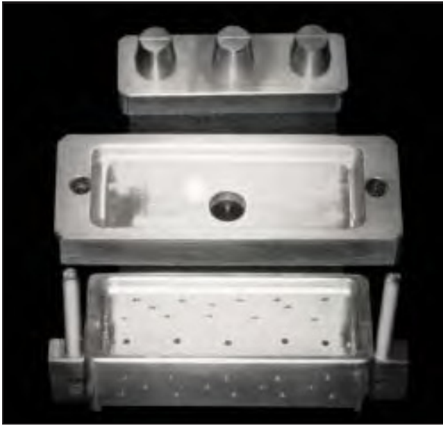
Fig 1 Metal master cast containing three full crown-abutment preparations, perforated custom metal tray, and metal index device.
